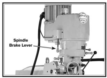
Figure 42. Location of the spindle brake lever.
